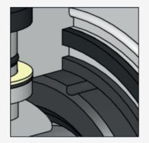
Fugitive emissions design according to ISO 15848 and TA LUFT / VDI 2440 reducing the potentially emission to the environment, the hydrogen losses and the risk of ignition.
