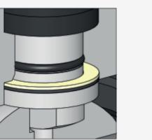
Anti-static device ensures the electrical conductivity between body, end, ball and stem according to European directive 2014/34/EU (ATEX)
