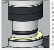
High purity hydrogen is an important requirement in some processes to guarantee high levels of quality and process performance and eficiency while keeping the valve with the firesafe safe design. To perform this the valves are designed with double insulation system where the first line is made from inert polymeric materials isolating the hydrogen media from any contact with graphite parts. This design is capable to avoid any contamination ensuring the high purity levels of the processes.
