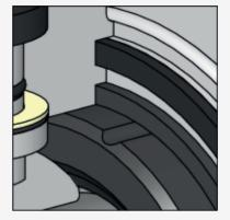
Firesafe design according to ISO 10497 and API 607 for critical services. Primary layer of TFE prevents graphite contamination into the media assuring the cleanliness of the processes. A metal backseat system allows the sealing in the event of a fire ensuring the tightness of the process.
