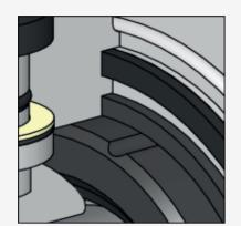
Double encapsulated body seals for extra resistance and tightness performance
