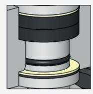
Explosive Decompression (ED) or Rapid Gas Decompression (RGD) is a failure mechanism associated with high pressure gas media. High pressure gas can reach easily the o'ring chambers. When the pressure is released, as when the valve is closed, the remaining gas located in the chamber expands causing fissures and o'ring failure.
