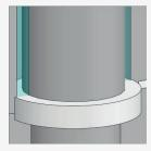
The expansion chamber allows the formation of a barrier or an insulation column of vapour between the liquefied gas and the packing increasing its performance and life cycle.
