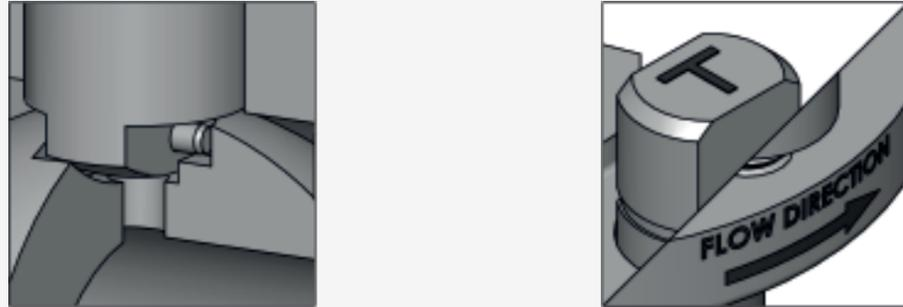
Rib and groove design between the ball and stem to guarantee the correct alignment of the upstream relief hole avoiding incorrect installations and possible malfunctions during the utilization. Once the valve is installed, the position of the upstream relief hole can be checked at any time through the top stem marking of the current position of the ball. The valve has also a flow direction identification for full integrated information.
